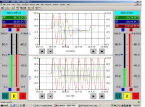
Left: When MFA (top) and PID (bottom) start from the same oscillating control condition, PID will continue to oscillate while the MFA will quickly adapt to an excellent control condition.
