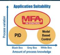
MFA is suitable for Grey box problems, where the process has uncertainties including load, fuel, and dynamic changes. PID – one algorithm for all, MBC – one algorithm fits one system, MFA – one algorithm solves one control problem.
