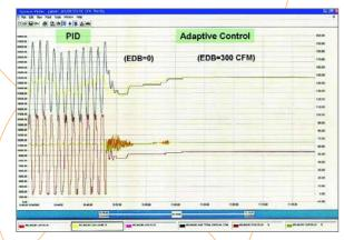
Actual comparison data between PID and Adaptive Control for air flow control at air handler, displayed in Dynamic Plotter at customer site.
