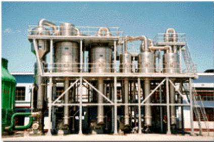
A multivariable MFA controller in CyboCon software quickly and tightly controls density and level by manipulating inflow and outflow simultaneously. An MFA constraint controller protects the evaporator level from running too high or too low.
