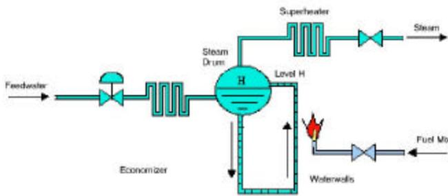
*This 1-Element/3-Element Drum Level MFA Control System can be easily launched to control the drum level when there are large disturbances in steam load, feedwater flow and fuel mix flow.*
