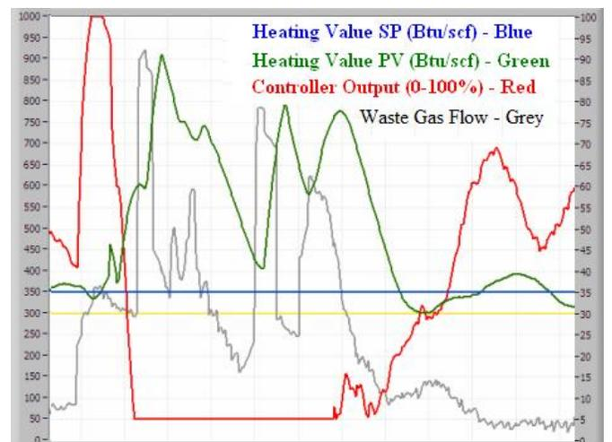
**Flare Process:** Most refinery and chemical plants operate flares to burn off waste gas. The vent gas heating value of a flare must be monitored and controlled based on EPA 40CFR60.18 rules.
