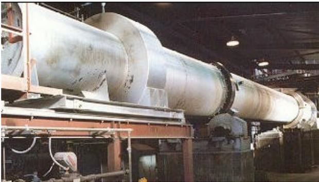
*An Anti-delay MFA controller with feedforward and robust functions manipulates coal flow intelligently to achieve tight kiln temp (blue) control.*
