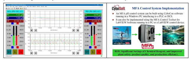
An MFA pH control system can be built using CyboCon software running on a Windows PC, interfacing to a PLC or DCS. It can also be implemented with the MFA Control Toolset for LabVIEW software, running on a LabVIEW control device.
