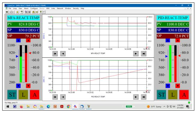
Typically, a non-self-regulating or runaway process like this could potentially be controlled using a high-gain P-controller. However, when the process also has a large time delay, controlling it becomes extremely difficult. A runaway process requires rapid control action in order to quickly reach a new balance point, while a process with a large time delay requires a more patient control action. These two control requirements are in conflict.
